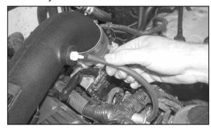
24. Install the provided vacuum hose onto the fuel pressure regulator and then onto the K&N® intake tube as shown.
