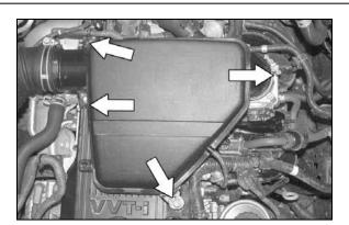
4. Remove the three bolts shown that secure the intake plenum to the engine and loosen the throttle body hose clamp.
