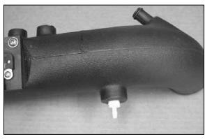
21. Install the supplied npt fitting into the K&N® intake tube as shown.
