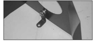
9. Install the small heat shield mounting bracket (070812) with the provided spacer onto the heat shield as shown.
