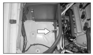
12. Install the heat shield onto the vehicle and secure with the provided hardware and nut removed in step #11.
