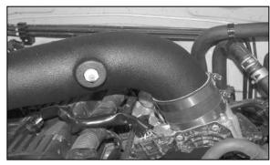
22. Install the K&N® intake tube onto the throttle body and align with the saddle bracket.
