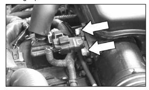
3. Remove the two bolts that secure the pressure sensor to the stock intake tube.
