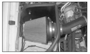
29. Install the  $K\&N^{\otimes}$  air filter onto the intake tube as shown.
