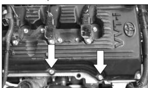
14. Remove the two valve cover bolts shown. **NOTE: These bolts will be reused.**
