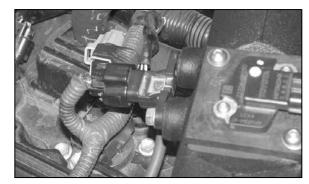
26. Install the pressure sensor onto the K&N® intake tube using the bolts removed in step #3.
